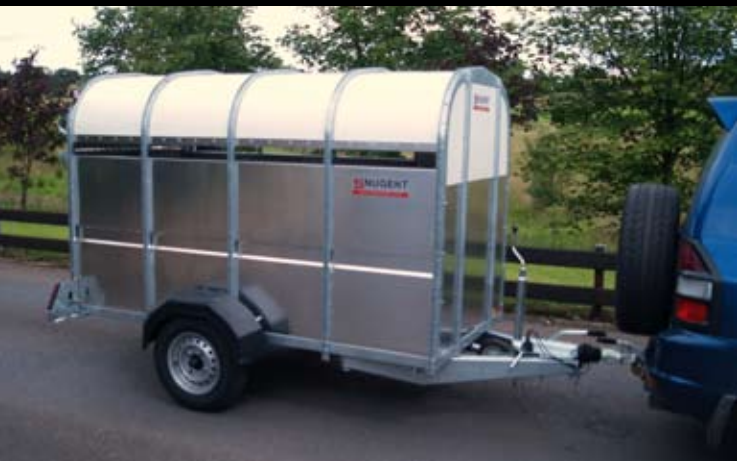
Single Axle Livestock Trailer with side vents.
